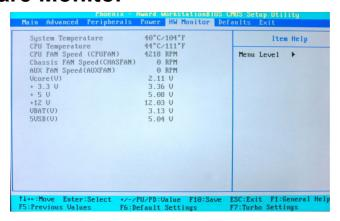
This menu is for monitoring the system status such as temperature, voltage, and so on.
