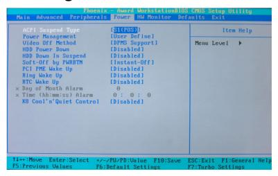
The Power Management Setup Menu allows you to configure your system to utilize energy conservation features as well as power-up/ power-down options.
