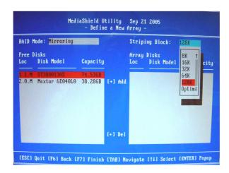
Next, in the "Free Disks" section, you can use the up/down arrow keys to select disks to be used in your RAID array. After highlighting a disk, use the right-arrow key to activate the disk as part of the RAID Array. The selected disk will move over to the "Array Disks" section. You can use the left-arrow key to reverse your selection. After you finish selecting all your disks, Press <F7>. A confirmation message will display as shown below. Then press <Y> to complete the RAID array creation.
