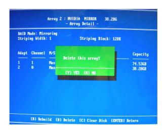
After the array is successfully deleted, the screen will display as shown below.
