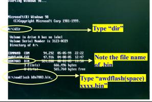
8. The initial AWARD BIOS FLASH screen (shown below-left) will appear and prompt you with the message, "Do you want to save BIOS?" Type "N" (Note: Typing "Y" is only used when saving the BIOS from the onboard BIOS to the floppy disk).
