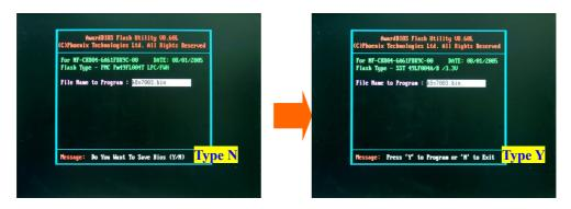
The next screen (shown above-right) will display a message "Press 'Y' to Program or 'N' to Exit". Then type 'Y' to begin the onboard BIOS flash procedure.
