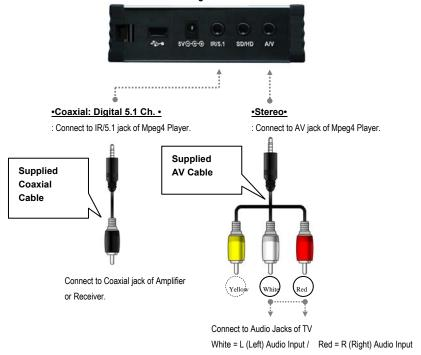
✓ When you can not hear sound after connecting Coaxial Cable, you have to change audio setup of Mpeg4 Player as Encoded Digital. See "2.2.2 Audio Setup"
