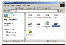
✓If new volume is not be appeared, check HDD format or not. and HDD file system. Windows 2000, XP detect both FAT32 and NTFS file system. Or connect power cable of Mpeg4 Player. 3) After copying data, remove Mpeg4 Player with using remove icon at Windows right-down corner. If you don't follow this procedure, data and Mpeg4 Player may have damage.
