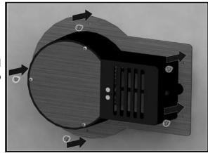
Tear this page off and cut the rectangle out. Then place on the duct work in desired position and trace the rectangle. Drill holes as indicated and then use a jig saw or metal cutting snips to cut out the rectangle.
