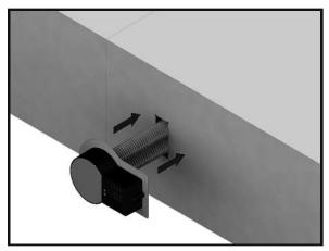
Step 5 Insert unit into pre-cut hole.
