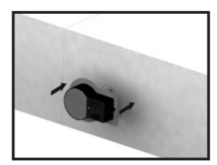
Step 3 Insert unit into pre-cut hole.
