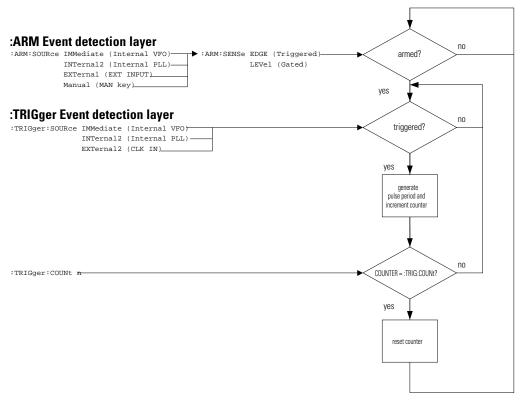
You program the comprehensive triggering capabilities of the instrument using the SCPI :ARM and :TRIGger subsystems. Using these two command subsystems you can program the operating modes of the instrument, which are set up using the Mode/Trigger screen on the front panel.
