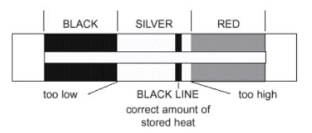
The heat indicator is above the roasting oven door and has three sections: black, silver and red. When the indicator is on or about the black line in the silver section, the range is at the correct working temperature. The purpose of the heat indicator is to show whether the range contains the full amount of stored heat and it should, therefore, only be referred to first thing in the morning or after a period of several hours during which no cooking has been done.
