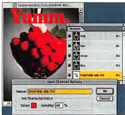
Photoshop's Spot-Color Channels When you ⌘-click on the New Channel button, Photoshop lets you specify a spot color and its solidity value.
