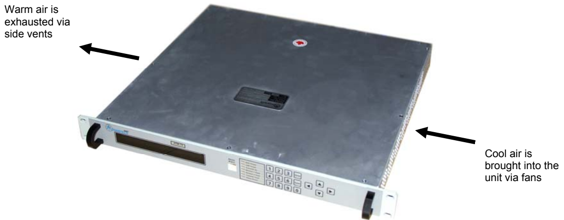
Figure 2.2: Air Path through the Enclosure
