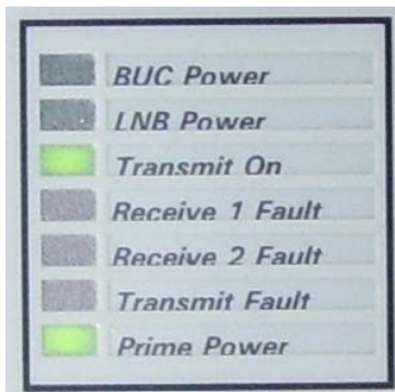
Figure 1.3: Front Panel LED Indicators
