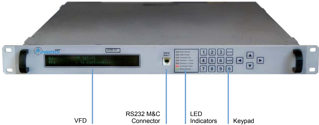
Figure 1.2: SBD75e Demodulator Front Panel
