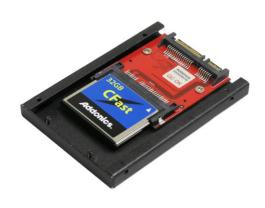
3.5" hdd mounting bracket for ADCFASTHDD (AA35HDBKT-SHCF)
