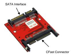
The unique CFast - SATA HDD Adapter is designed to enable CFast media to be used as a direct replacement for a 2.5" SATA hard drive. As a result, any equipment, such as Notebook computer, that uses a 2.5" SATA hard drive can be easily converted to use the low power and shock resistant CFast media. Once installed, the CFast appears as an ordinary hard drive to any OS and can be configured as a boot device.
