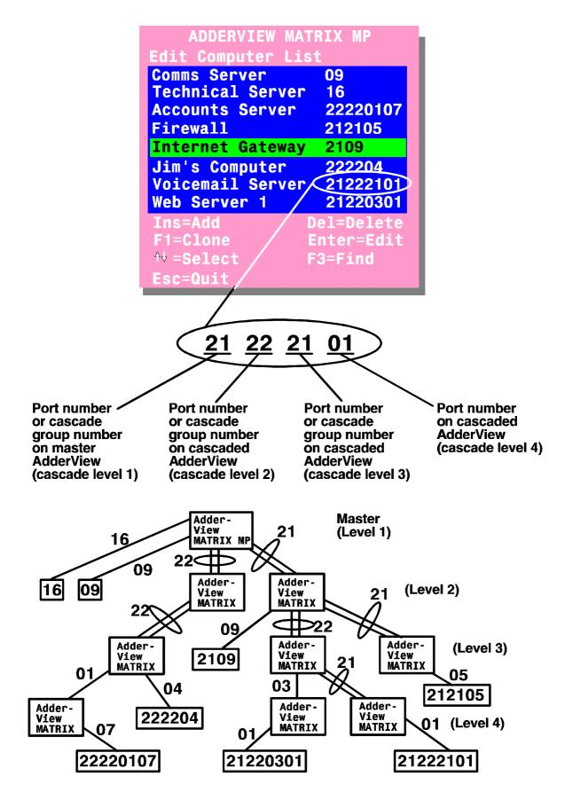
Fig. 6 - Creating menu entries for computers that are connected to cascaded AdderViews
