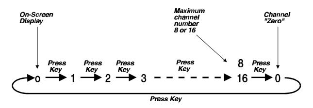
Action of the COMPUTER key if the front panel controls are enabled, security has been set and the current logged in user only has access to computer ports 1,3 and 7
