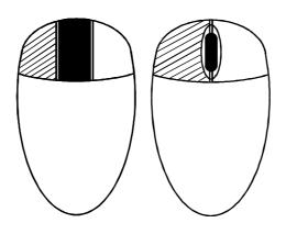
Hold down centre button ( ) Press and release left hand button ( ) to select next computer
