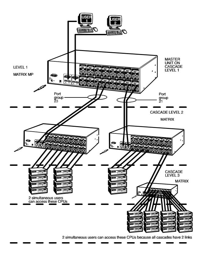
Fig. 5 - A cascaded application using multiple AdderView MATRIX units
