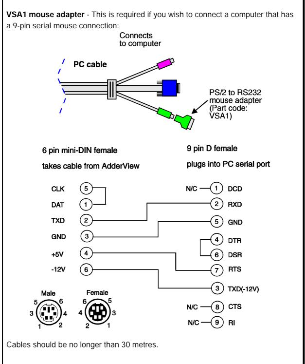
NOTE - There are several common wiring specifications for 6-pin mini-DIN to 9-pin serial adapters. If you have an adapter that has been supplied with a mouse it may have a completely different internal wiring to that shown above and may not be compatible with the AdderView MATRIX MP **VSA2 keyboard adapter** - If your PC has a 5-pin DIN AT style keyboard connector you will need a PS/2 to AT keyboard adapter 6-pin mini-DIN female to 5-pin DIN male.
