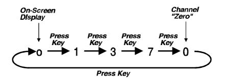
Action of the COMPUTER key if the front panel controls have been disable.
