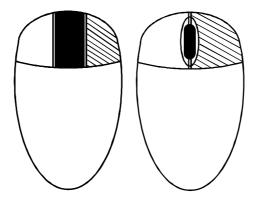
Hold down centre button ( ). Press and release left hand button ( ) to launch the on-screen menu
