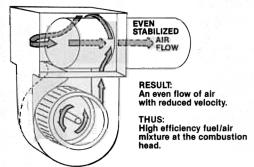
Patented Turbo-Reversed-Air System or TRA, the major breakthrough that accounts for INTERburner's fuel economy. Inside each INTERburner, TRA stabilizes dynamic pressure while maintaining high static pressure. It creates the most uniform airflow at the combustion head and gives
