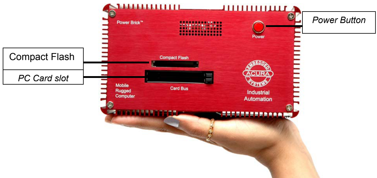
Figure 2.2: Front side of PowerBrick
