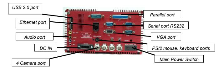
Figure 2.2: Back side of PowerBrick-CV.
