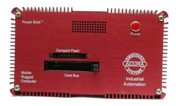
Figure 2.1: Front side of PowerBrick-CV.
