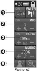
Figure 10: (1) Radio transmission band display, (2) Microphone volume display, (3) Adjustable Echo time display, (4) Adjustable volume control, (5) Singing mode switch (stereo).
