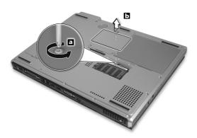
3 Insert the memory module diagonally in the slot (a), and then press down gently until it clicks in place (b).
