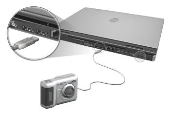
USB is plug and play, which means you can connect and start using a USB device without having to restart your computer. You can also disconnect the device at any time.
