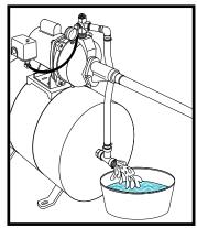
for pump to prime. **Failure to prime in 5 minutes:** Stop motor, remove pressure gauge plug from discharge tee, add more water, try again. Allow pump to run long enough to clear the well of sand or dirt and to insure well will not run dry. Stop motor.
