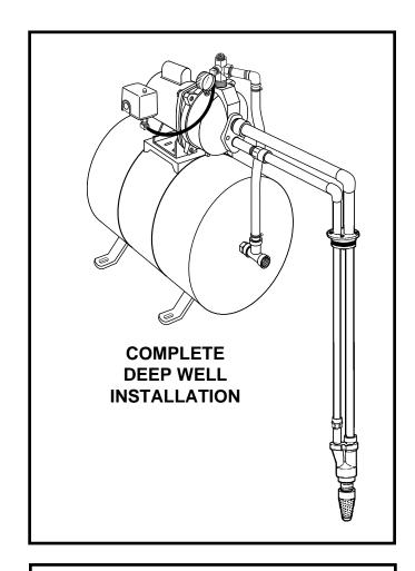
**CAUTION:** If you change pressure switch settings, set the cut-off pressure low enough to shut off the pump. The recommended pressure is 2 PSI below your pump cut-off pressure. Example: if a 20-40 PSI pressure switch is being used, tank pressure should be 18 PSI. If a valve shuts off and the cut-off setting is too high, the pump will run continuously without water flow causing overheating and serious damage.
