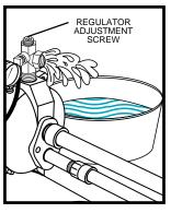
ed without pressure dropping to zero. If pressure falls completely, retighten adjustment screw and re-adjust. Steady pressure must not be less than 24 lbs. for the R520 and 32 lbs. for the R100. If no pressure shows: Stop motor, remove pressure gauge plug from pressure regulator, add more water, and try again. Complete installation should look like the drawing to the right.
