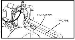
1-1/4" PVC pipe needed to connect the 1" female PVC adapter and the 1-1/4" male PVC adapter to the 1" and 1-1/4" PVC elbows. The diaphragm pressure tank is factory preset to 30 PSI. Reset the pressure to 18 PSI using a tire gauge. This is vital to the proper operation of the system. Remove pressure gauge plug.
