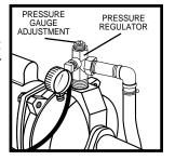
STEP 9 maximum water flow is obtained without pressure dropping to zero. If pressure falls completely, retighten adjustment screw and read-just. Steady pressure must not be less than 24 lbs. for the R520. If no pressure shows:
