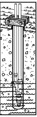
**STEP** Remove pipe clamp and slide well seal #RWS4-1012 over PVC pipes and onto well casing. DO NOT let assembly slide down into well. Position assembly so that twelve inches of PVC pipes protrude from well seal. Using crescent wrench, turn
