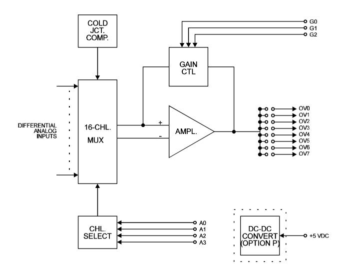
Figure 1-1: AIM-16 Block Diagram
