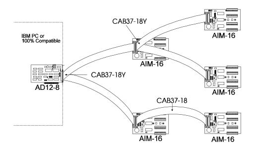
Figure 2-1: Use of CAB-37Y Cables
