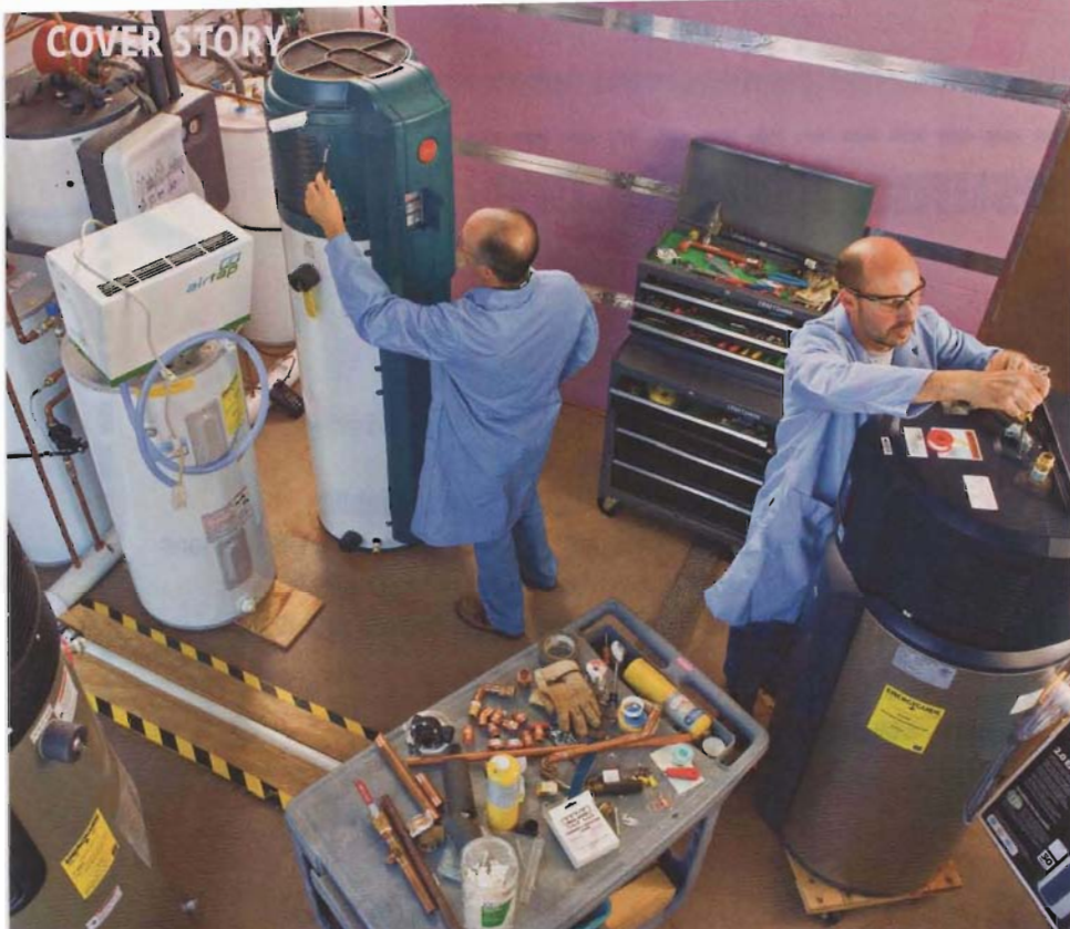
GAUGING SAVINGS Testers prepare to put hybrid heaters from Rheem and GE through their paces.
