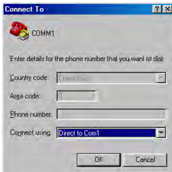
Figure 2-3 Configure the port for connection
